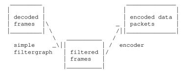
Simple filtergraphs are configured with the per-stream -filter option (with -vf and -af aliases for video and audio respectively). A simple filtergraph for video can look for example like this:
